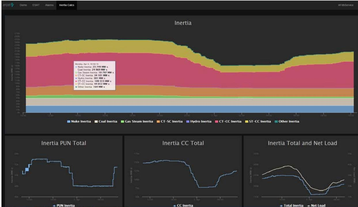
**Figure 3.2: ERCOT Dashboard to monitor real-time inertia**
